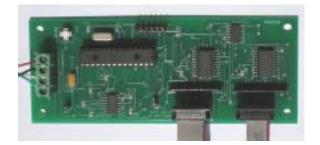
The system consists of a small pc board (shown above) and a main board. The small board mounts inside the Aiphone NHX control unit and connects to connectors CN8 and CN9. The main board is in a cabinet mounted nearby.
